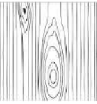
Natural small dark knots present, as well as healthy knots and cat paw.
