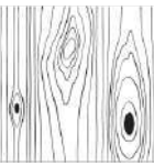
Country dark knots and filled cracks up to 2 mm in width can be present.
